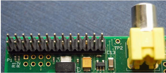
These pins are a physical interface between the Pi and the outside world. At the simplest level, you can think of them as switches that you can turn on or off (**input**) or that the Pi can turn on or off (**output**). Seventeen of the 26 pins are GPIO pins; the others are power or ground pins.
