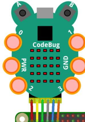
The CodeBug can be tethered to the Pi and then programmed using Python.
