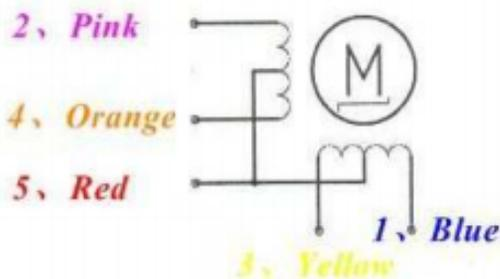
We use a driver board which we can control from the Pi. This way we can reverse the current and turn the motor in both directions.
