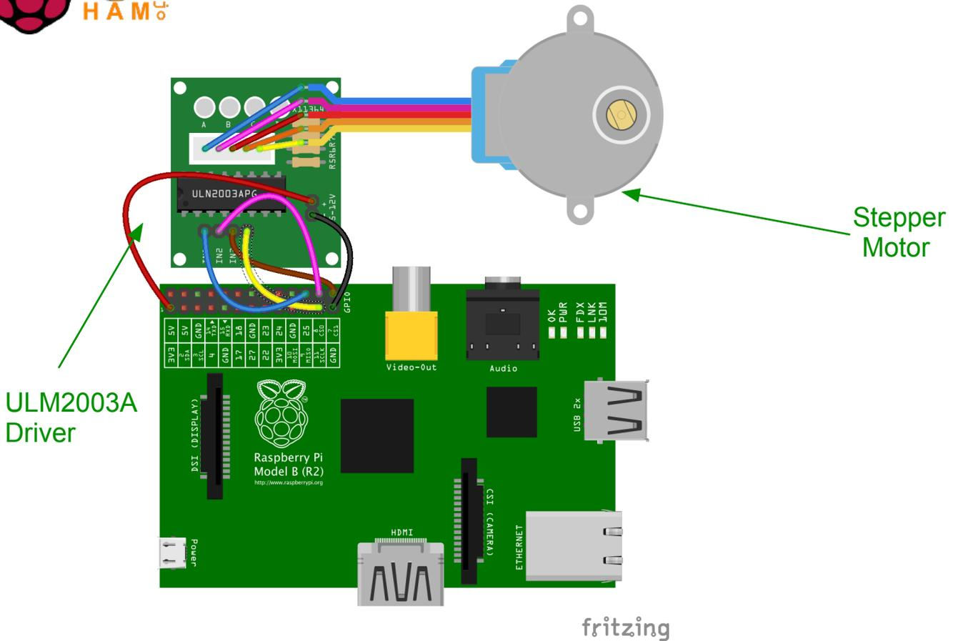
Stepper motors are DC motors that move in steps. They have multiple coils that are organised in groups called "phases". By energising each phase in sequence, the motor will rotate, one step at a time.
