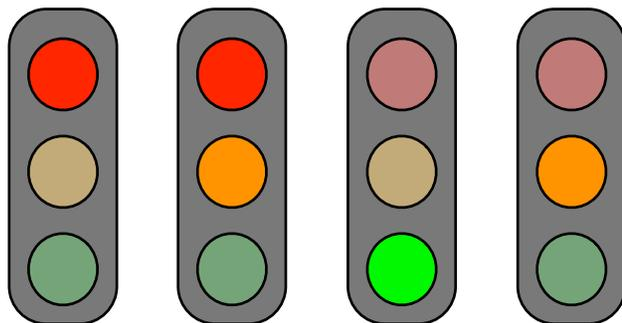
Remember the STOP (red) and GO (green) cycles should be longer than the GET READY (when amber is on).
