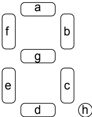
So by turning on a, b, c, d, e, and f, we can make a zero
