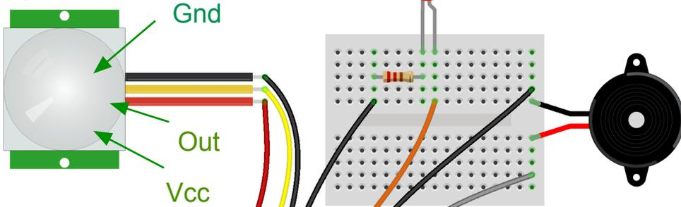
This time we're using the +5 volts pin. **Make sure you connect it to the correct pin on the sensor!**
