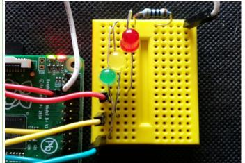
GPIO pins **7**, **15**, and **23** can be coded to supply power to their corresponding LED. All 3 LEDs share the same resistor and ground pin **6**.
